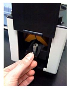
4) Transmission/Absorbance/Reflectance readings will significantly change once the Praying Mantis is installed (Transmission/Reflectance will go down; Absorbance will go up)
